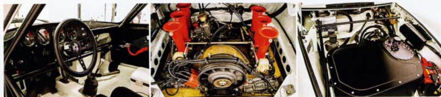
Below, left to right: The first Andial retains its spartan RSR interior. Its 3.0-liter engine sports a host of power tricks. A racing fuel cell fills up the trunk.
