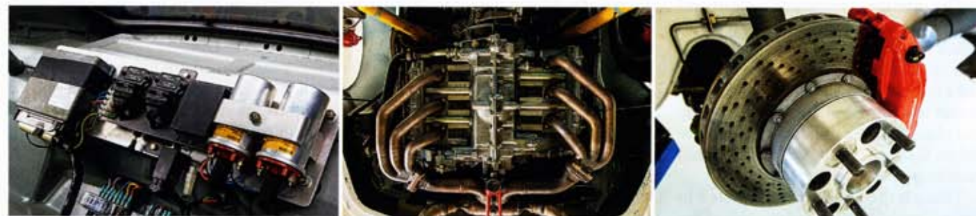
Below, left to right: The last Andial's electrics are mounted to the bulkhead. Its 3.6-liter flat six sports 993 headers. 993 Turbo brakes are almost too big.
