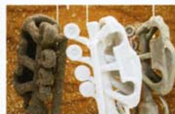
Three invested waxes in various states of layering. The white one is ready for the kiln.
