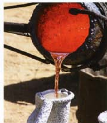
Molten bronze is poured into the investment casing.
