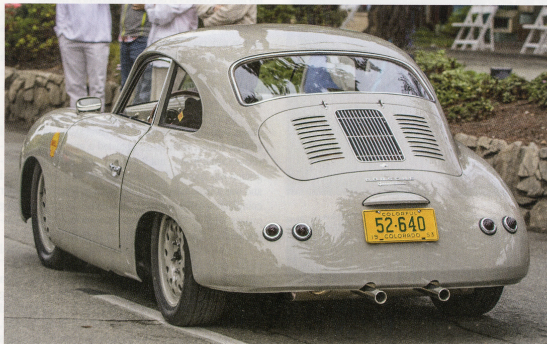
No junk in this trunk. Custom fuel tank and filler neck are polished aluminum, as are the access covers. The right side cover opens to a storage compartment. Below: Louvered deck has 911R style hinges and a button release. Side windows are lexan.
