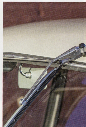
Wiper motor is mounted just behind the windshield. It drives the right arm, which in turn drives the left with an old-school exterior connecting link.
