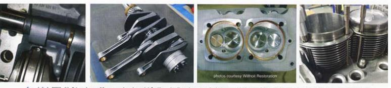
From left: In Willhoit's 2.1 engine an 82 mm crank and special Carillo rods allows just enough clearance with the cam lobes. Wider cylinders required a new sealing solution to the specially-shaped combustion chamber with twin plugs. Durabar cylinders and short-skirt 3 ring pistons with a custom dome and exhaust valve pocket.
