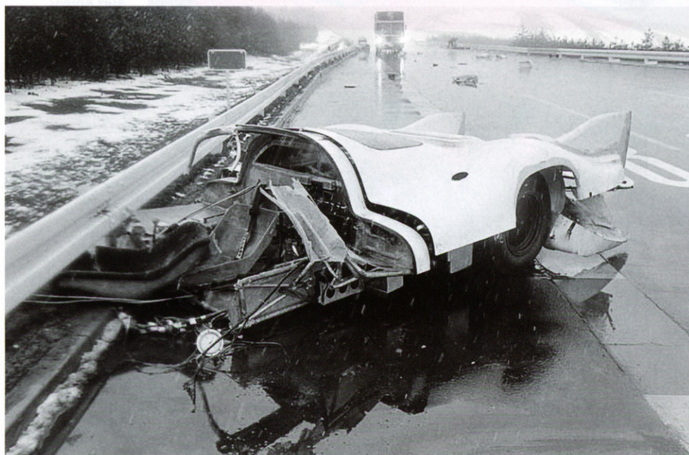
Below: The aerodynamic configuration of the original 917 was unstable, as demonstrated by Kurt Ahrens' crash during testing at Ehra-Lessien.
