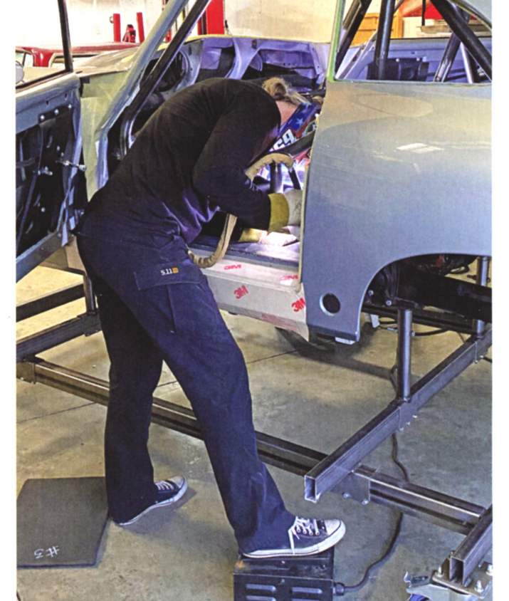
Above left: This is just one of many lists Pedro and Nicola composed to ready the car for La Carrera. Above right: Campuzano welds up the car's roll cage.
