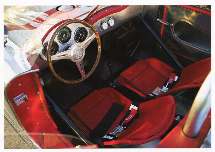
Besides engineer ing chassis and shaping bodies, Runge also designs, patterns, and sews custom interiors for comfort and driving efficiency. This one features dual rally stopwatches.
