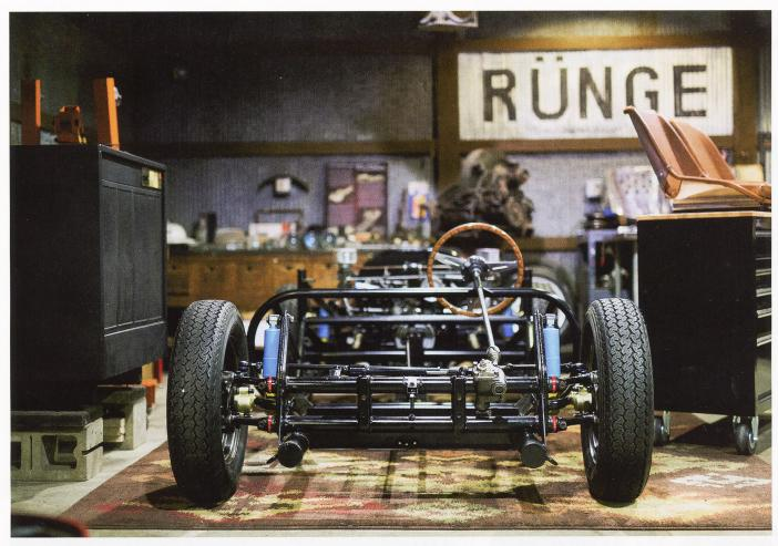
Although his first chassis was based on a scavenged Formula Vee, Runge has since progressed to self-designed two-seaters. With every iteration, he's learned to make them stiffer and stronger with better handling while maintaining the "contemporary vintage racer" concept.
